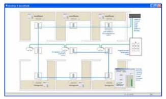
Customized graphics and personal dimming controls for individual level or facility level control.
